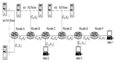
Figure 4.The multiple congestion network topology for simulation
