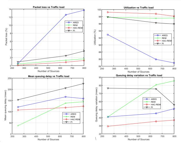
Figure 6. The changes of network parameters when the number of loads change
