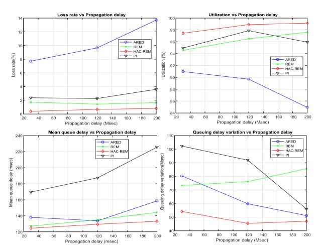
Figure 8. The changes of network parameters when RTT change
